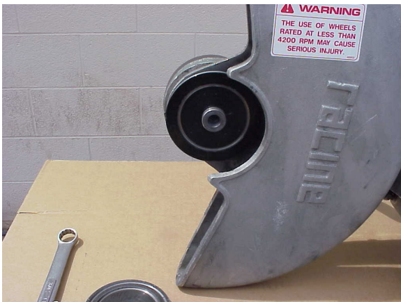
Inner Flange Installed
