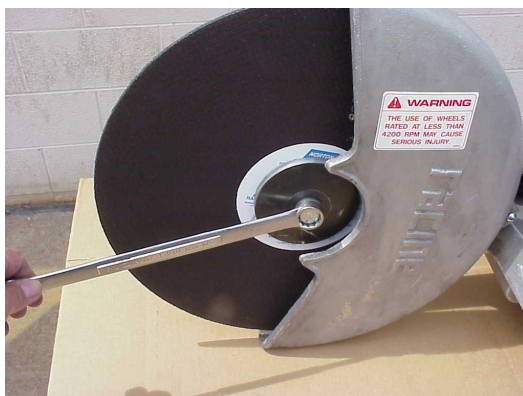
Outer Flange Installed
